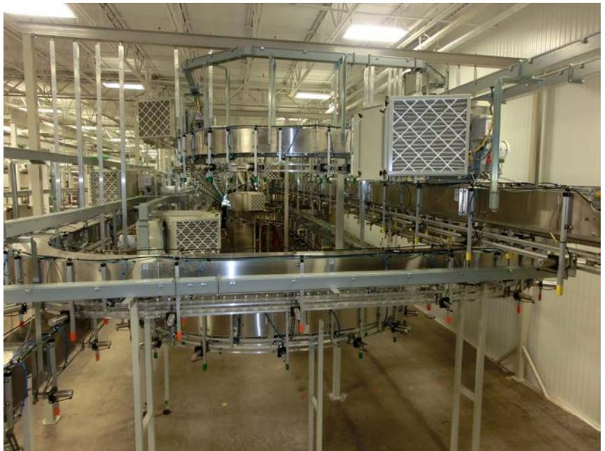
exits the louvers or nozzles at 4,000 to 10,000 fpm. Louvers are common because they can be easily and inexpensively stamped into sheet metal. Louver size, spacing, and the number of rows vary based on application. Conveyors for denser items such as scrap material typically have louvers with larger openings to handle the high volume of air it takes to float and push dense items.
