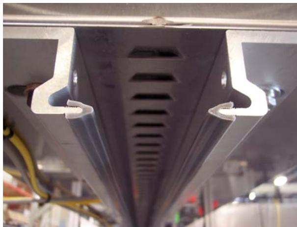
on these conveyors are held within low-friction guides to keep them oriented. A less common version, the hybrid air conveyor, uses two plenums. Air flows through louvers to an inner plenum in which items such as metal scrap are moved. Internal air conveyors are limited to lengths of about 100 ft. or less due to pressure losses within a pipe. Hybrid conveyors can be virtually any length because air enters and vents along its entire length.
