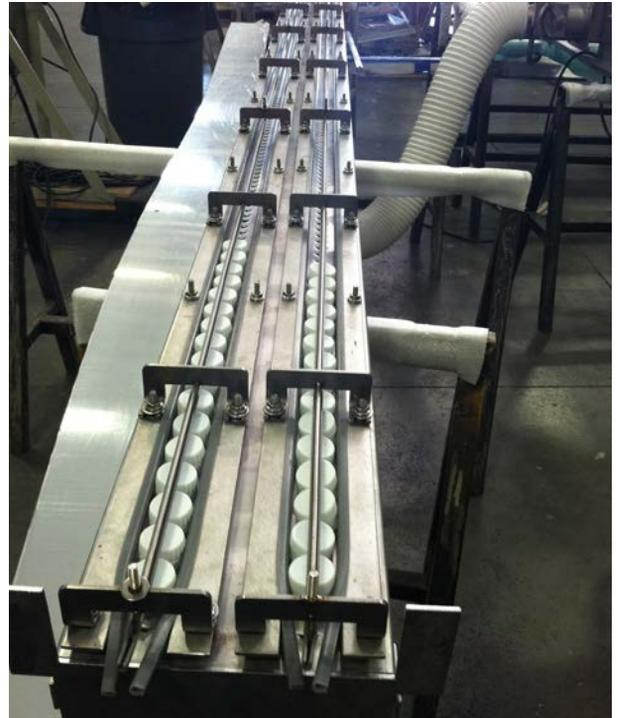
machining centers and recycling sites are perfect applications for air conveyors because the long ribbons of scrap metal easily snag and are razor-sharp.
